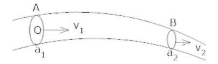
Let a<sub>1</sub>, a<sub>2</sub> = area of cross – section at A and B
